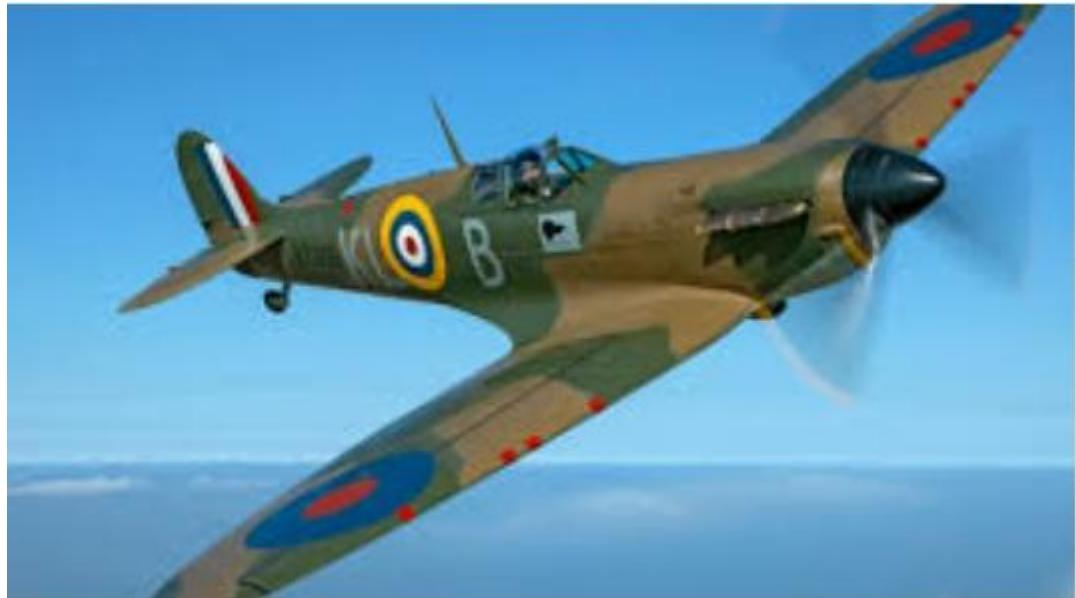
Chris Clarke noted that the RR Merlin engine in the Spitfire was a V12 carburettor engine, which would splutter in a dive, and the only safe way to dive was to roll onto its side. The enemy Messerschmitt had primitive fuel injection in its Mercedes Benz
